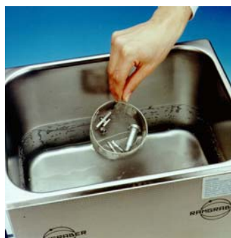
Cleaning of dispensing needles with ZESTRON® ES 200 in an ultrasonic tank
